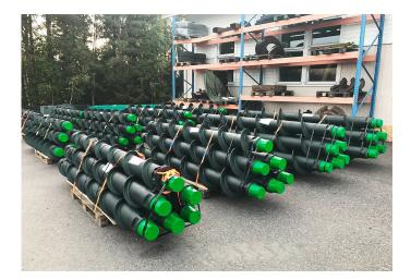
GEONEX is manufacturing Auger Rods especially designed for Horizontal drilling for the most common casing sizes (139,7-1220 mm). Normally, the Auger rods are manufactured 3,0 m or 6,0 m long with API Reg connections. Thread types of other standards or with HEX rod ends are possible. We can also design Auger rods after your demands. We can repair or replace the screw blades on existing drill rods.
