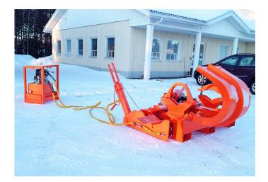
The Break out Bench is a great help when servicing, maintaining and repairing a DTH-hammer. The Break out Bench is operated hydraulically. The hydraulic power can be produced by some mobile device such as a Wheel Loader, or the Bench could be equipped with the Geonex Power Pack. Geonex manufactures two different break-out bench models.
