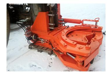
GEONEX Clamps enable better controlling of pile pipe during drilling. This is needed especially in difficult ground conditions and special situations. Clamps can be also equipped with tool break out drill rod connections. Clamp set also insures that pipe is correctly aligned to rotary head.
