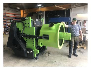
Geonex Rotary Heads are engineered for DTH-Drilling. Design is compact and strong Engineered for both horizontal and vertical drilling. Rotary head can be mounted straight to feed carriage or as an option, there is also possibility for tilt function with cuttings collector. Speed switching valve option and different motor sizes also enables drilling of large diameter range. Rotary head has in-built air swivel with large hole through.
