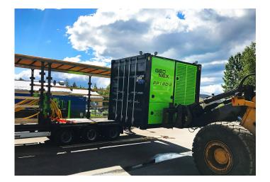
PP180 is a robust power pack for demanding jobsite conditions. Power pack is very service friendly unit with a lot of room to work and also additional space for storing tools. Two open circuit variable displacement hydraulic pumps combined with radio controlled directional valves can provide hydraulic power for HZR610, HZR1000 and to many other various applications. Tier 4 Final diesel engine meets all modern emission requirements.
