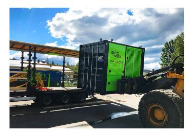
PP180 is a robust power pack for demanding jobsite conditions. Power pack is very service friendly unit with a lot of room to work and also additional space for storing tools. Two open circuit variable displacement hydraulic pumps combined with radio controlled directional valves can provide hydraulic power for HZR610, HZR1000 and to many other various applications. Tier 4 Final diesel engine meets all modern emission requirements.
