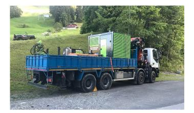
The PP180HA hydraulic and compressor unit is very compact and mobile. It provides all that is needed for drilling small diameter casings from Ø139.7 -219.1 mm with HZR220. Even though the PP180HA is primarily engineered to serve HZR220, it can also be usedin other applications also, where there is need for hydraulic and pneumatic power.
